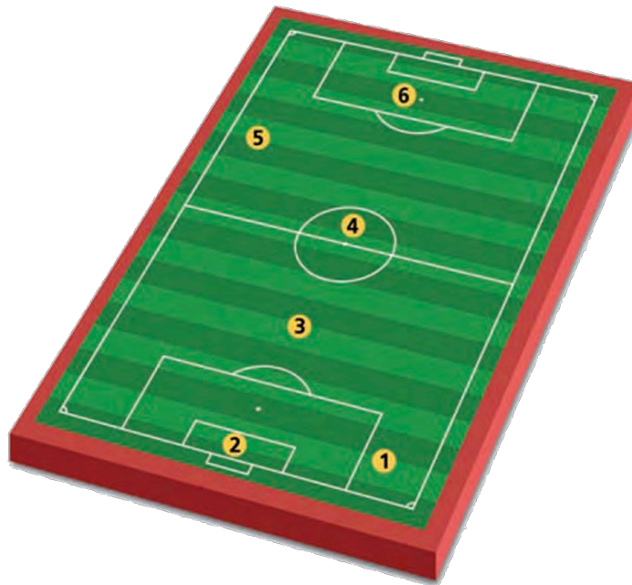
FIFA measuring points for ball roll test
