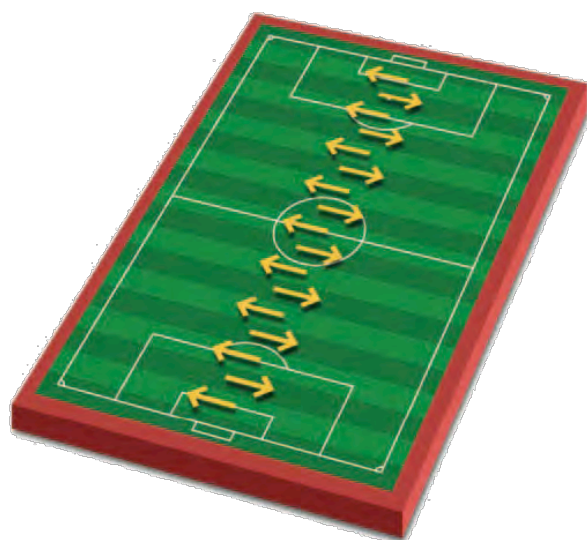
Direction the rolls have been installed in.
