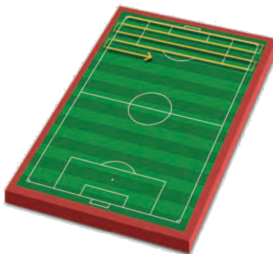
Direction of travel for maintenance to ensure the fibres stand upright.
