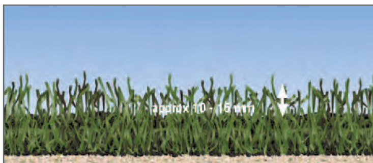
Pile projection length for texturised fibres
