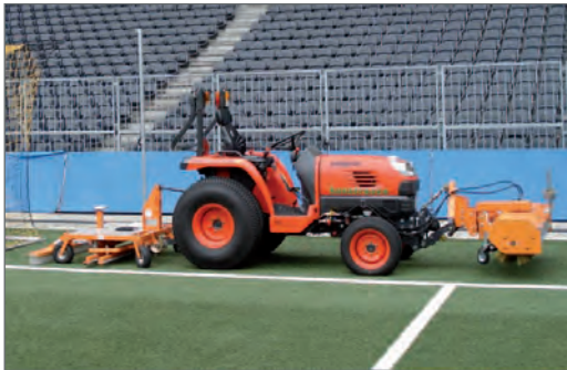
Unit with fixed brush and needle bars
