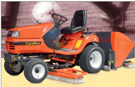
Rear mounted oscillating suspended brushers
